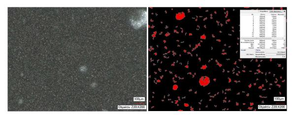
In the second example, the solid lubricant particles are evenly and homogeneously distributed in the grease matrix. The size and distribution of the agglomerates corresponds to the defined limits of the QM.
